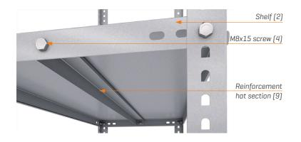
If the aim is to increase the load-bearing capacity of the shelves (2), longitudinal reinforcements (9) can be fitted under the shelves and fastened in position by an M8x15 screw (4) at each end.
