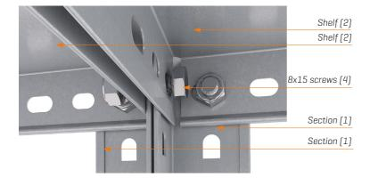
The modules are connected to each other by matching the sections [1] and adjacent shelves [2] and fastening them with an M8x15 screw [4].
