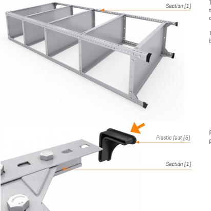
Then, position the remaining two sections (1), fastening them to the panels (2) as described, using the corresponding screws.
