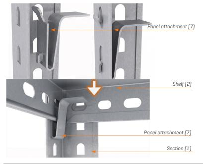
The conventional system of fastening the shelves in position using screws can be replaced by fitting panel attachments on the sections.
