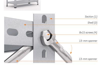
Tighten the screws using two 13-mm spanners, taking care to keep the shelf vertical and level in the required location.
