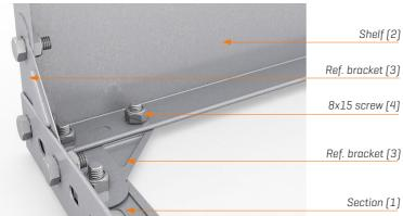
The reinforcement brackets are to be fitted between the shelves [2] and the sections [1] on both sides, as shown in the attached illustration. They are fastened in place with M8x15 screws [4] using the corresponding holes and manually tightening them in such a way as to allow the joint a certain amount of give.
