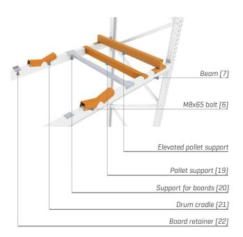
Depending on the particular use of each storage system, different components can be fitted to the beams thereby adapting the loading levels to receive specific types of goods and operate with a given handling system.
