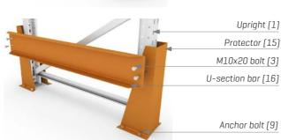
For full frame protection, a U-section bar [16] should be connected to the lateral faces of the upright protectors [15] using four M10x20 bolts [3].
