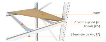
or boards can be fitted with the aid of Z beam supports [25], as specified in the project design.
