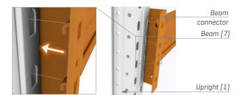
The basic structure is produced by attaching the beams [7] to the frames.
