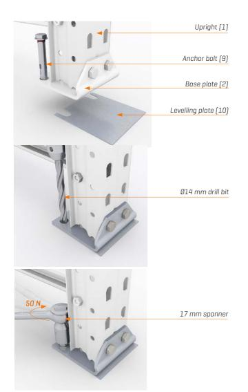
The uprights [1] have to be fixed to the floor to increase the structure's safety. If the foundation surface is uneven, then levelling plates [10] must be introduced below the base plates [2] to ensure the structure is levelled and plumbed correctly.
