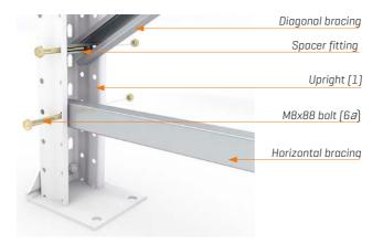
All of the bracing elements are attached to the frame with their open faces towards the inside of the upright [1] and their ends are secured with spacer fittings to prevent any free movement.
