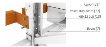
They are positioned just above the beams [7] for each loading level.
