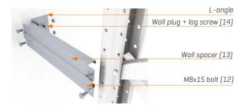
When specified in the storage system's design plans, wall spacers [13] should also be installed. These consist of an L-angle and frame spacer [11] that are connected together using four M8x15 bolts [12] and subsequently secured to the wall using a wall plug and lag screw [14].
