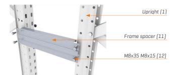
Attach the spacers (11) to the sides of the uprights (1) using four M8x15 bolts (12) placed as close as possible to the nodes connecting two diagonal bracings.
