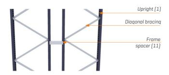
When installing double rows, they must be joined together using frame spacers [11].
