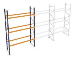
Then attach the rest of the beams [7] until all the levels are in place, thus completing the assembly of the initial module
