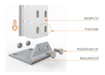
Attach the base plate [2] to each upright [1] using two M10x20 bolts [3] with their respective nuts.
