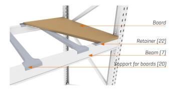
or boards can be fitted with the aid of the supports [20] specified in the project design, plus four retainers [22] per level.
