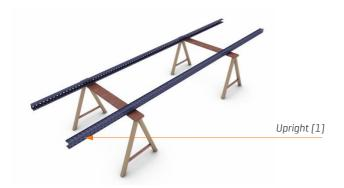
Place the two uprights [1] in parallel and with their open sides facing each other, either on some supports or directly on the floor.
