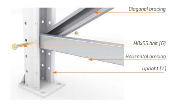
Position the first horizontal [4] and diagonal bracings [5] with their open sides facing each other, then secure them to the upright with a M8x65 bolt [6].
