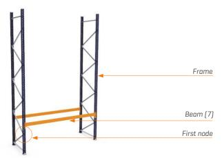
Place the structure in an upright position and attach the first two beams [7] at the height of the first loading level.
