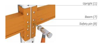
Once fitted correctly, beam connectors are secured using safety pins [8]. These are fully inserted into their correct position with a few light blows from a hammer.
