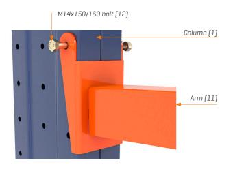
The arm (11) is fastened to the column using a M14x150 or M14x160 bolt (12) depending on the width.
