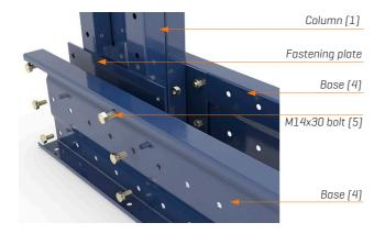
Bolt the end of the bases to the fastening plates on the lower side of each column using six M14x30 bolts [5].
