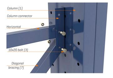
The diagonal [7] and horizontal [8] bracings are fastened to the connectors on the sides of the columns using M10x20 bolts [3].
