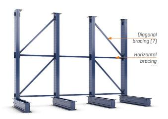
The standard composition of the vertical bracing, after it has been fastened to the columns, is as shown in the illustration.
