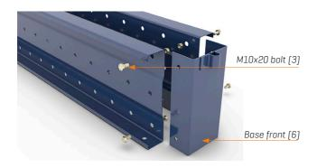
A base front [6] has to be fitted on the front of the bases to close off the edges of both bases; fasten it in position using M10x20 bolts [3].
