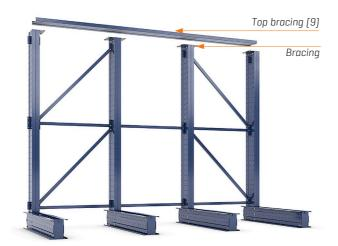
Columns of 3000 mm or higher must be coupled together using a top bracing [9] positioned horizontally on the ends.
