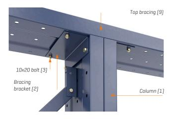
Then fasten it to the bracing frames using the M10x20 bolts [3] previously fitted to the columns as indicated in step 1.
