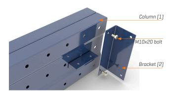
The coupling is made by fastening the narrowest side of the bracket to the column using two M10x20 bolts [3]. The edge of the column and the widest side of the bracket must be flush with each other.
