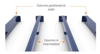
Columns of 3000 mm or higher have two bracing brackets fixed to the top ends, one on each side, except for those positioned at the ends of the structure, which have only one bracket.
