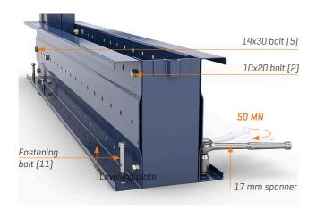
The bases must be levelled with metal levelling plates if necessary. Then, fully tighten the 10x20 bolts [2] on the base front as indicated in step 2.
