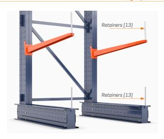
Cantilever shelving is often used to store goods which, owing to their physical characteristics and because they are not properly packaged or fastened in place, may move to the front of the arms and fall off the shelf. To avoid this, vertical retainers [13] can be fitted on the ends of the arms and bases.
