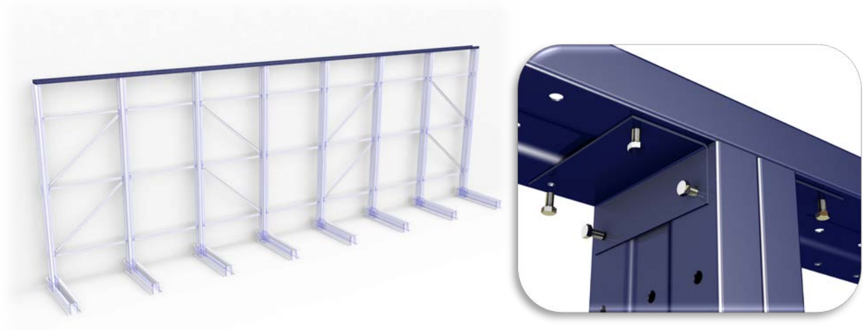
Diagram of the top bracings and details of their attachment using M10x20 bolts
