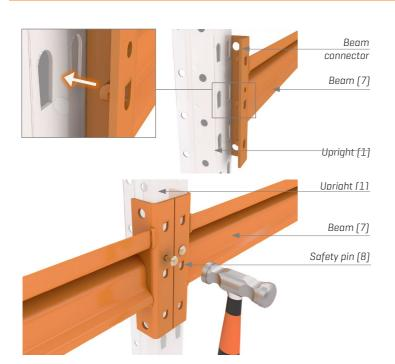
The basic structure is achieved by attaching the beams [7] to the bracings [1].
