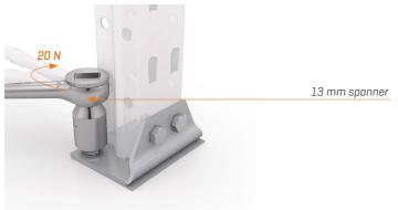
Finally, screw the bolt down until it is secured firmly in position. Apply a recommended tightening torque of 20 Nm.
