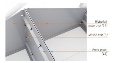
Finally, the remaining dividers should be distributed based on user requirements.
