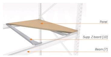
or boards, with the Z beam supports (10), as specified in the project design.
