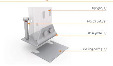
The uprights (1) have to be fixed to the floor to increase the structure's safety. If the foundation surface is uneven, then levelling plates (14) must be introduced below the base plates (2) to ensure the structure is levelled and plumbed correctly.
