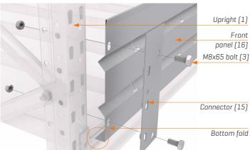
Place the connector with two or three hooks (depending on the type of panel) in the front holes on the upright.
