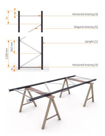
The diagram shows the correct positions of the diagonal [5] and horizontal bracings [4] on the frame.
