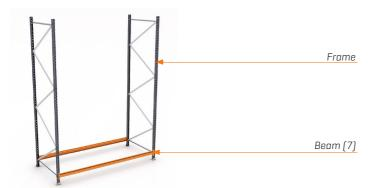
Place the structure in an upright position and attach the first two beams [7] at the height of the first loading level.
