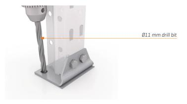
Drill a hole in the floor to a depth of at least 80 mm using a  $\emptyset 11$  mm bit.
