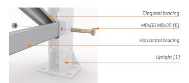
Position the first horizontal (4) and diagonal bracings (5) with their open sides facing each other, then secure them to the upright with a M8x35 bolt (6).
