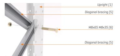
Next, place the remaining diagonal bracings (5) with their open sides facing the same direction and again secure them M8x35 bolts (6).
