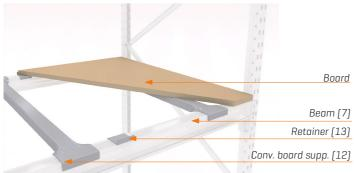
or boards, with conventional supports (12) as specified in the project design, plus four retainers (13) per level.
